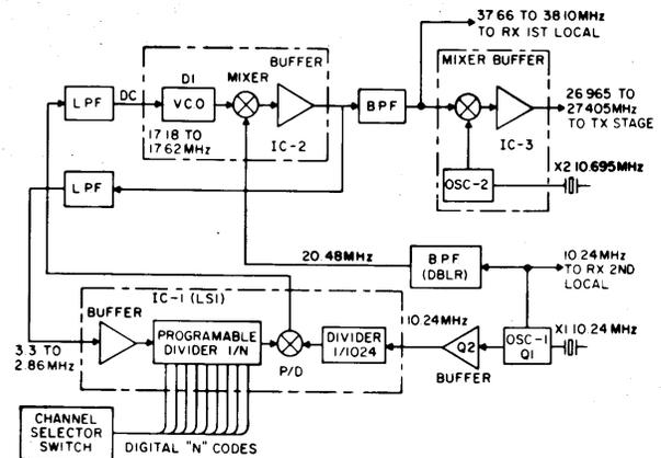
Figure 1 – PLL Block Diagram (except 14T305)
