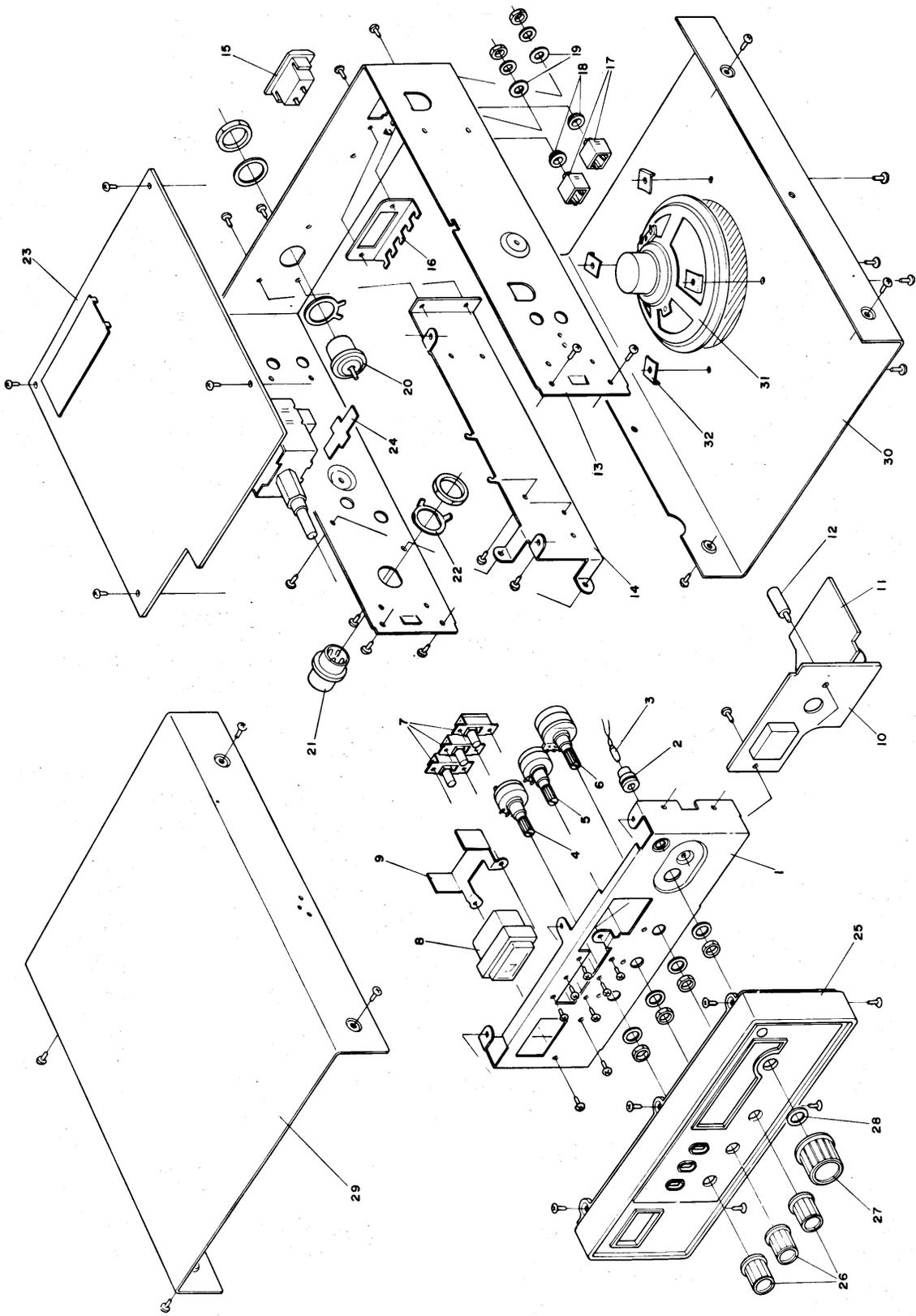
Figure 14 – Exploded View – Model 14T304
