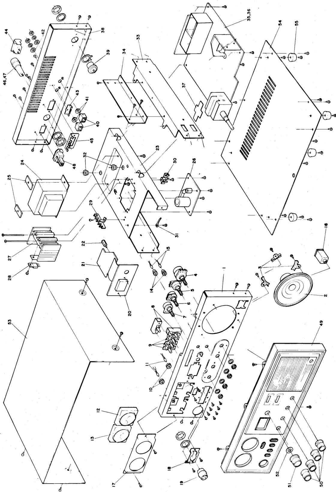
Figure 13 – Exploded View – Model 14T303
