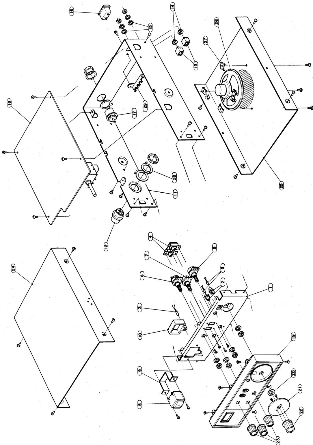
Figure 11 — Exploded View — Model 14T260
