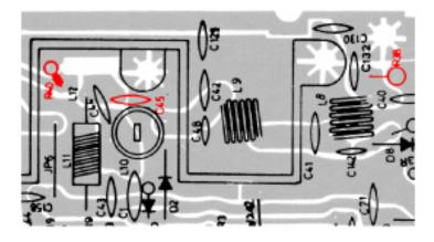
2) Install EKL Components' EN-1230 at R40. The EN-1230 is a POLARIZED part. Make sure that it is installed correctly with the positive lead toward L12.
