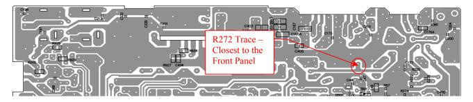
21) For S-9 Models Only – Do not perform this step on S-3 or S-6 models. Add a 1K ohm, <sup>1</sup>/<sub>4</sub> watt resistor across R214 on solder side of the radio PCB. See diagram below.
