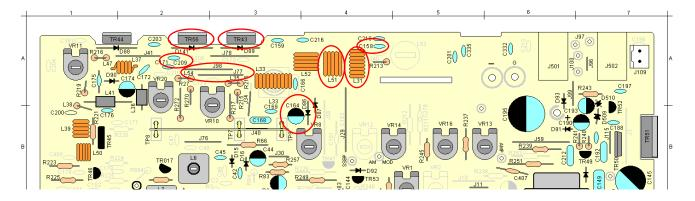
8) On the solder side of the radio PCB, remove C160 and C402. These parts are circled in red on the parts layout diagram below.
