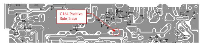
20) Locate the Blue wire from the RFX75 and route it through the slot on the transceiver's PCB where TR43 and TR56 were removed. On the solder side of the transceiver PCB, solder the Blue wire to the trace at R272 that is closest to the front panel of the transceiver. This location is +8 volts in transmit only. See diagram below.
