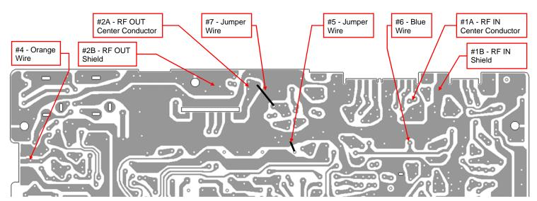
**Illustration B** – EPT3600\* Series PCB Solder Side Solder locations for wires in steps 1 through t.
