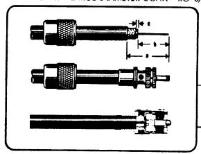
Cut end of cable even and strip jacket, braid, and dielectric to dimensions shown in table. Tin exposed center conductor and braid
