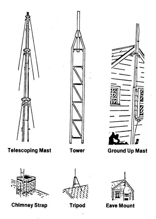
Although there are many variations to the examples, all appear to be simple — but don't believe it! If you are installing an antenna for the first time, please, for your own safety as well as others, seek professional assistance. Never use plastic pipe, conduit, wood poles or thin walled tubing. Use only masting that is specifically made for antenna support and has a length and wall thickness that is designed to carry the weight and wind load of your antenna.
