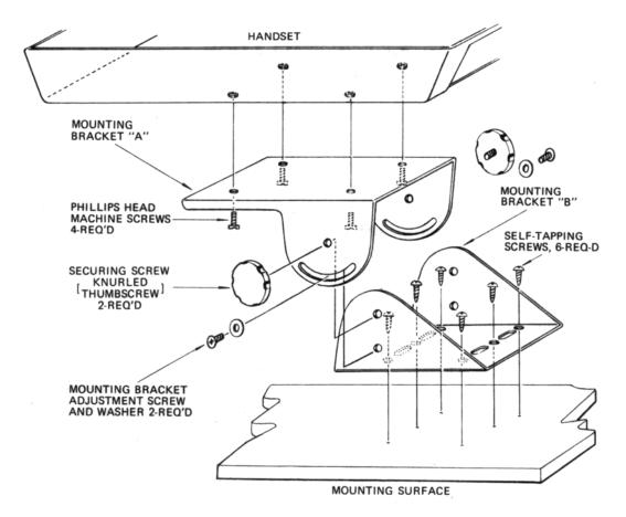
FIGURE 1. TRANSCEIVER MOUNTING, EXPLODED VIEW
