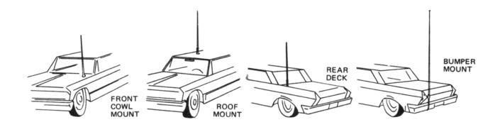
FIGURE 7. MOBILE ANTENNA MOUNTING
