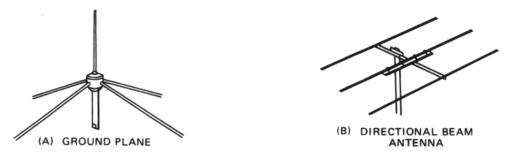
FIGURE 8. BASE STATION ANTENNAS
