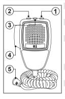
1 Up Button : Use this button to change the channels upward.
