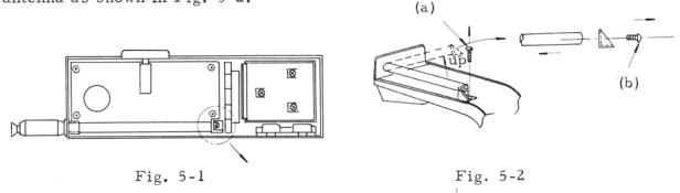
TO REMOVE BATTERY COMPARTMENT HOLDER, remove the three screws (a) on battery compartment holder.
