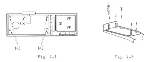
TO REMOVE THE PUSHBUTTON SWITCH, remove two screws (a) on the switch holder.
