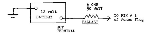
THE BALLAST RESISTOR should be mounted in the engine compartment since it will become hot.
