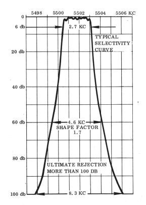
FIGURE 3. CRYSTAL FILTER CHARACTERISTICS
