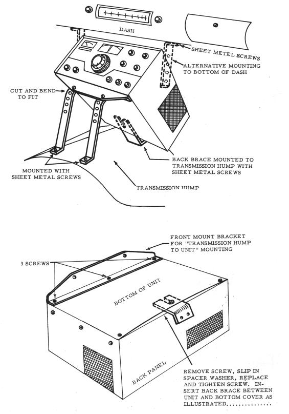
FIGURE 4. MOBILE INSTALLATION MOUNTING DETAILS
