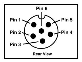
Warning: When wiring alternative microphones to this unit, Do Not short pin 6 to any other pins on the connector or damage to the unit may occur. Many service techs often short these pins to determine the mic wiring config. Shorting the 13.8VDC on pin 6 to other pins such as pin 4 may result in damage to the Microprocessor or Power Supply in the unit.
