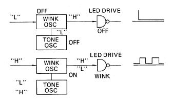
Figure 3. Operation of Wink Osc When Its Input Is "Low" and "High".
