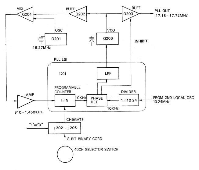
Figure 1. Block Diagram for PLL Synthesizer Circuit.
