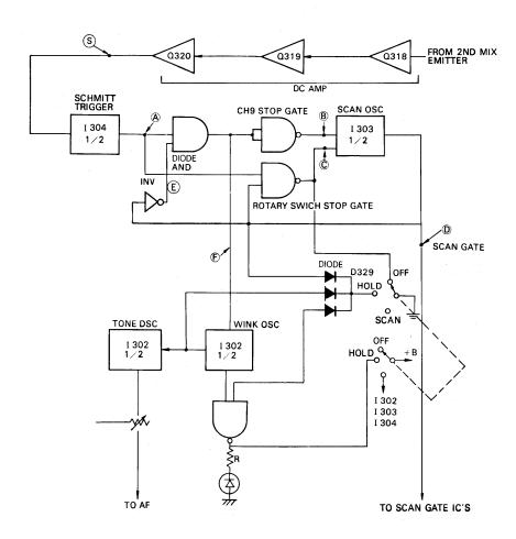
Figure 2. Block Diagram of Scan Circuit.
