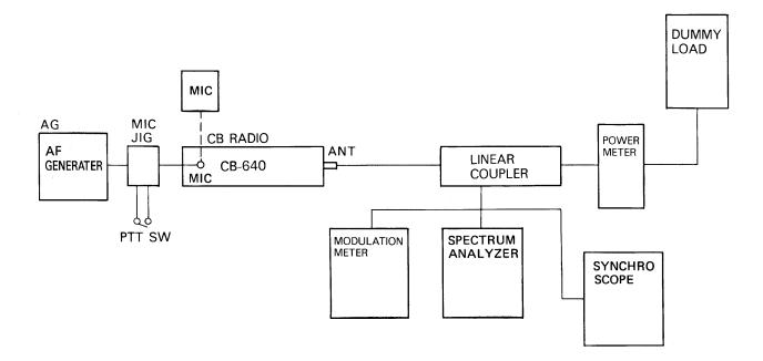
Figure 4. Interconnection for Adjusting the Transmitter Section.
