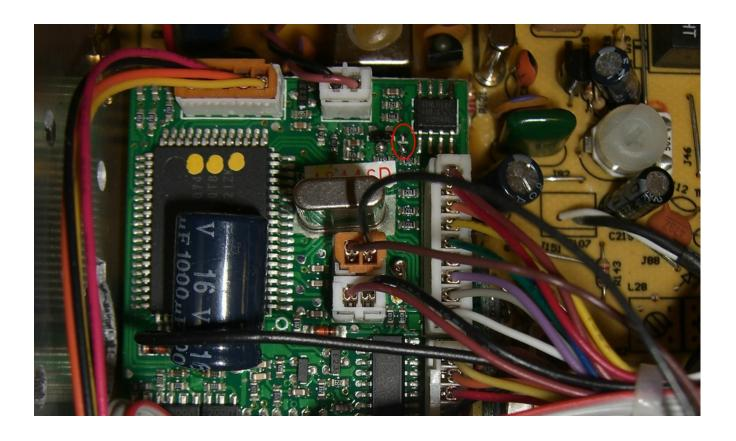
Solder bridge the two pads that are shown above in the red circle. Bridging these pads is very easy using a soldering iron with a fine tip.
