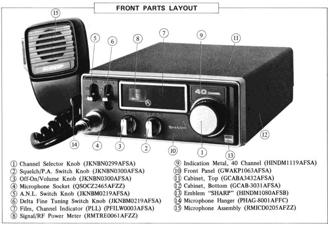
Figure 8 FRONT PARTS LAYOUT
