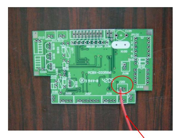
The red wire (which is originally connected to first lead of IC-358 of the module board mounted on PCBX-0335R3) is to be connected to the left hole of J-201 on the PCBX-0335R6.
