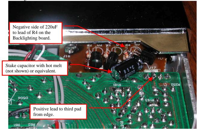
Figure 2: Installing the 220uF Capacitor
