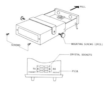
NOTE: WHILE CHASSIS IS OPEN BE CAREFUL NOT TO DISTURB ANY COIL ASSEMBLIES, AS THEY MAY AFFECT CRITICAL ALIGN-MENT WITHIN THE SET.
