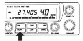
To stop automatic scanning, press **SCAN** again. **SCAN** disappears from the display.
