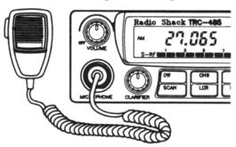
Press MODE to select the mode of operation — AM, LSB (Lower Side Band), or USB (Upper Side Band). (See "Notes on SSB Reception" on Page 13.)
