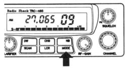
Rotate CHANNEL to select a channel.
