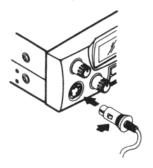
2. Slide the microphone onto the microphone holder.
