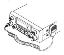
Caution: To disconnect the microphone from the transceiver, press the tab on the side of the plug. Then pull out the plug. Never pull on the microphone cable.
