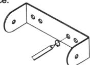
In each marked location, drill a hole slightly smaller than the supplied mounting screws.
