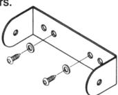
Attach the CB to the mounting bracket using the supplied rubber washers and mounting knobs.
