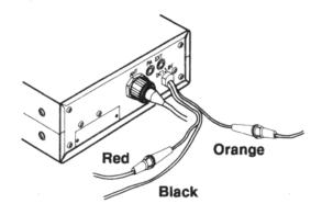
Connect the red wire (with an inline fuse holder) on the back of the transceiver to a point in your vehicle's fuse block that has power only when the ignition is in the ACC (accessory) or ON position. Connect the black wire to a metal part of the vehicle's frame (chassis ground).
