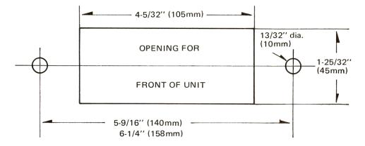
[As supplied, control shafts are separated 5-5/8" (142mm)]
