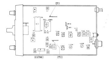
**NOTE**: Figure 1 provides test point and alignment location information.
