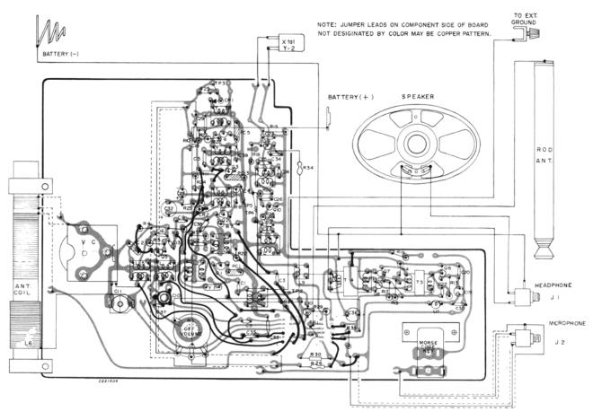
Component Location (Circuit Wiring)
