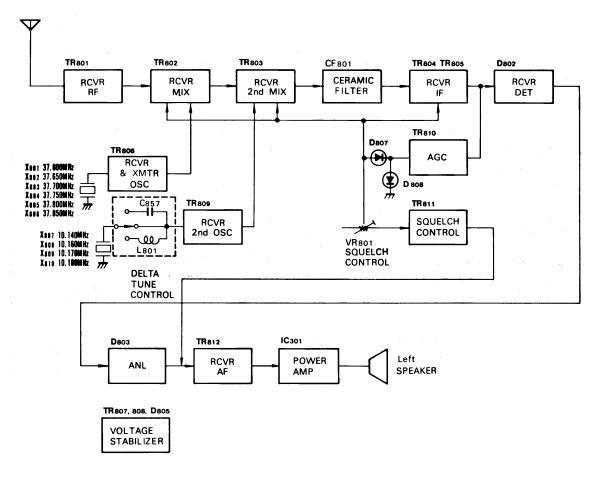
Figure 3. CB Receiver, Simplified Block Diagram
