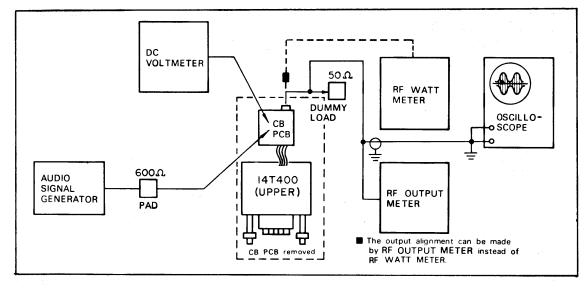
Figure 11. Test Connections for Alignment of the CB Transmitter Section
