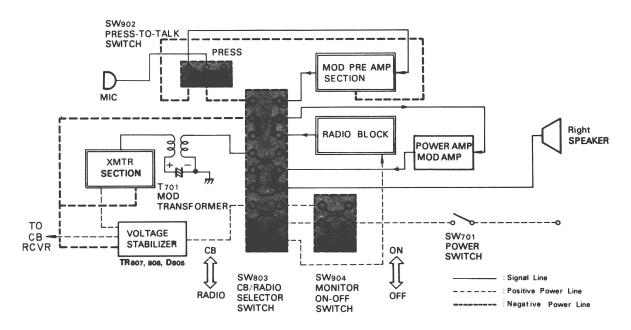
Figure 2. CB/Radio Selector Switching
