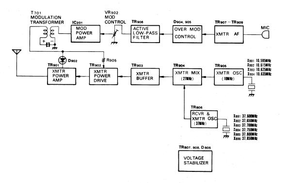
Figure 7. CB Transmitter, Simplified Block Diagram
