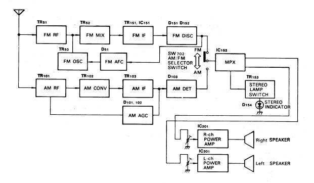
Figure 8. AM/FM/FM-Stereo Radio Simplified Block Diagram
