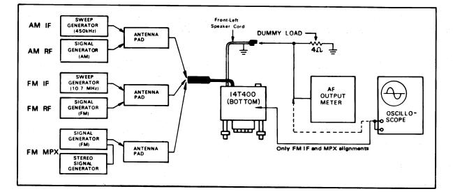
Figure 9. Test Connections for Alignment of the AM/FM/FM Radio
