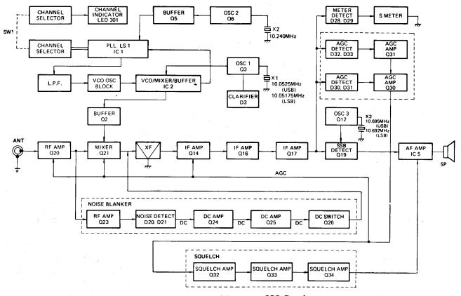
Figure 4 - Block Diagram - SSB Receive
