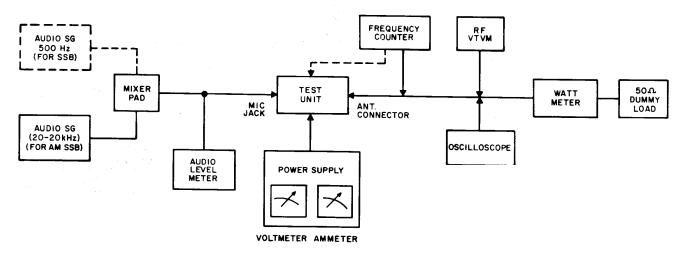
Figure 7 - Test Equipment Hook-Up - Transmitter
