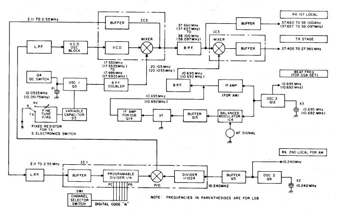
Figure 1 - PLL Block Diagram
