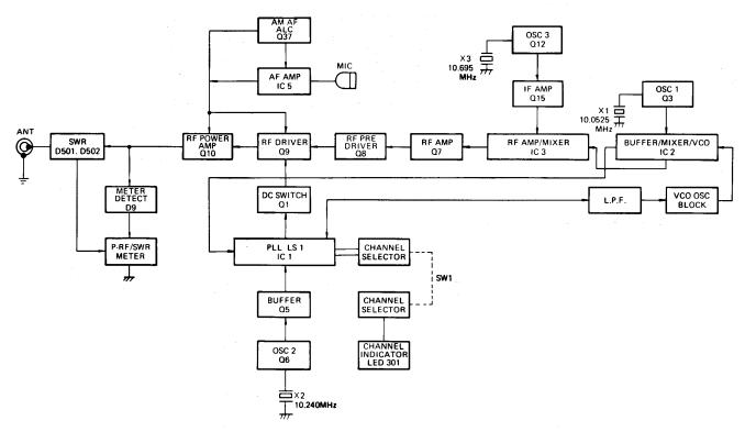
Figure 3 - Block Diagram - AM Transmit
