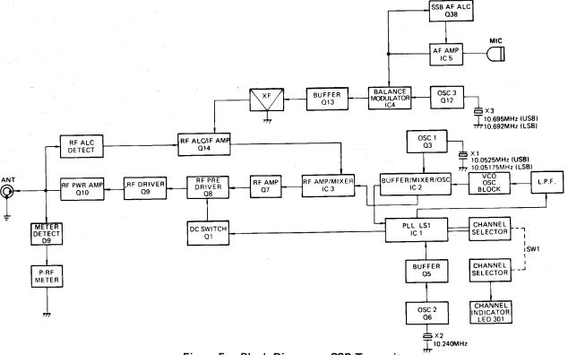
Figure 5 — Block Diagram — SSB Transmit
