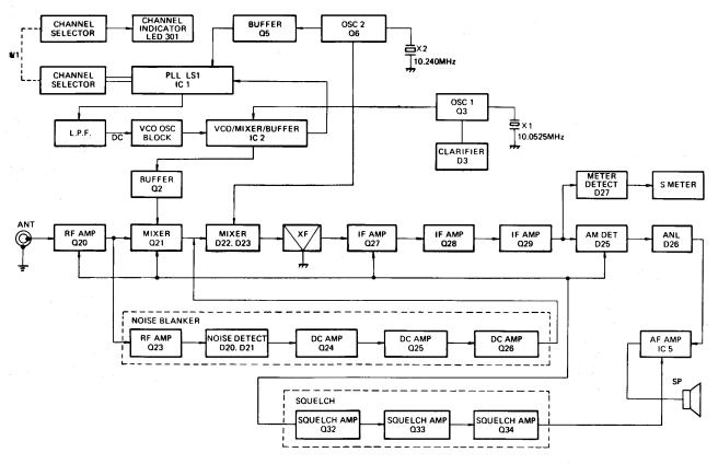
Figure 2 - Block Diagram - AM Receive
