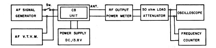
Figure 4 - Transmitter Alignment Test Equipment Set-Up
