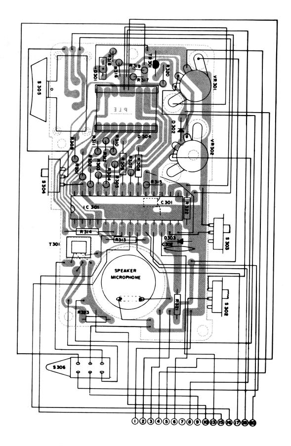
Figure 7 - Printed Board - Microphone/Speaker Assembly
