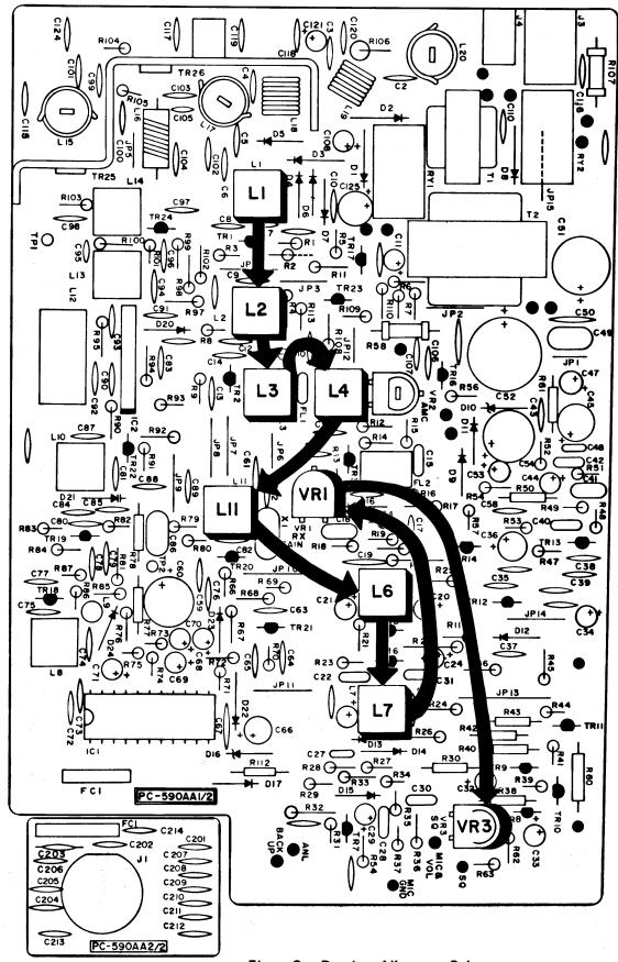
Figure 3 — Receiver Alignment Points
