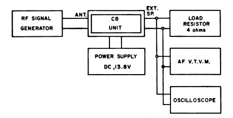
Figure 2 - Receiver Alignment Test Equipment Set-Up
