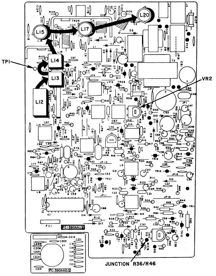
Figure 5 — Transmitter Alignment Points
