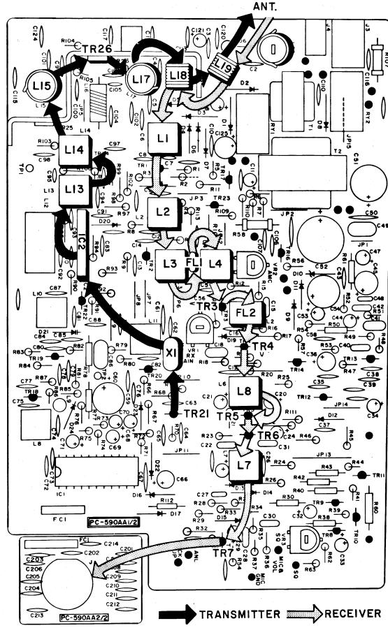
Figure 6 — Transceiver Signal Paths
