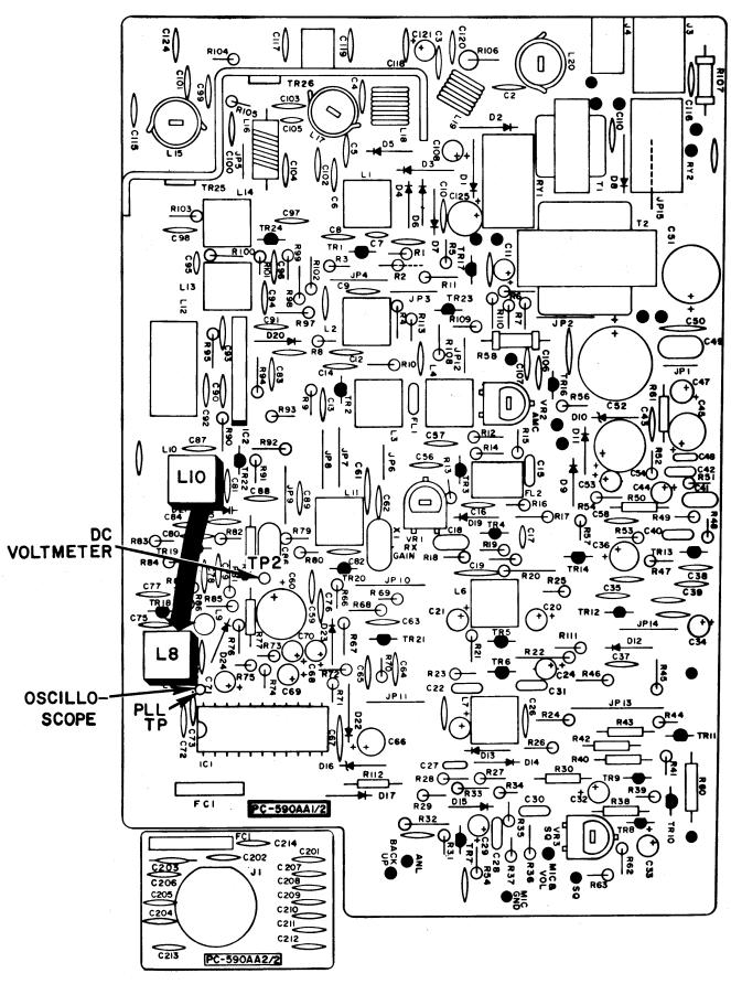
Figure 1 — PLL Alignment Points
