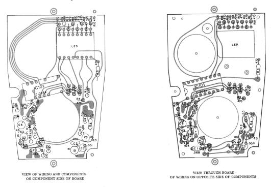
Figure 4. Mic/Speaker/Control Board (Foil on Both Sides)
