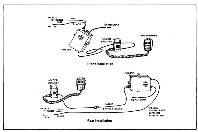
Figure 9. 14T275 Cable Interconnections
