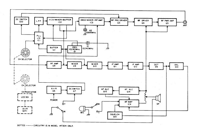
Figure 2 - Block Diagram for 14T260 & 14T304
