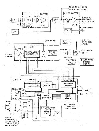
Figure 3 – PLL Block Diagram (14T305 only)
