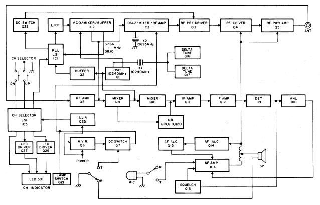
Figure 5 - Block Diagram for 14T305
