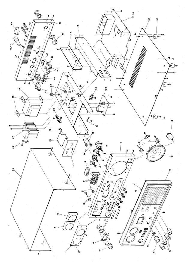
Figure 13 - Exploded View - Model 14T303
