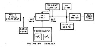
Figure 6 - Test Equipment Hook-Up
