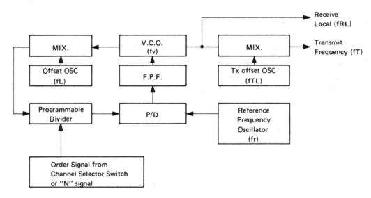
Fig. 5 Block Diagram of PLL Frequency Synthesizer Circuitry for CB transceiver
