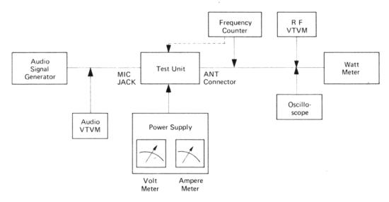
Fig. 6 Connections of test equipment
