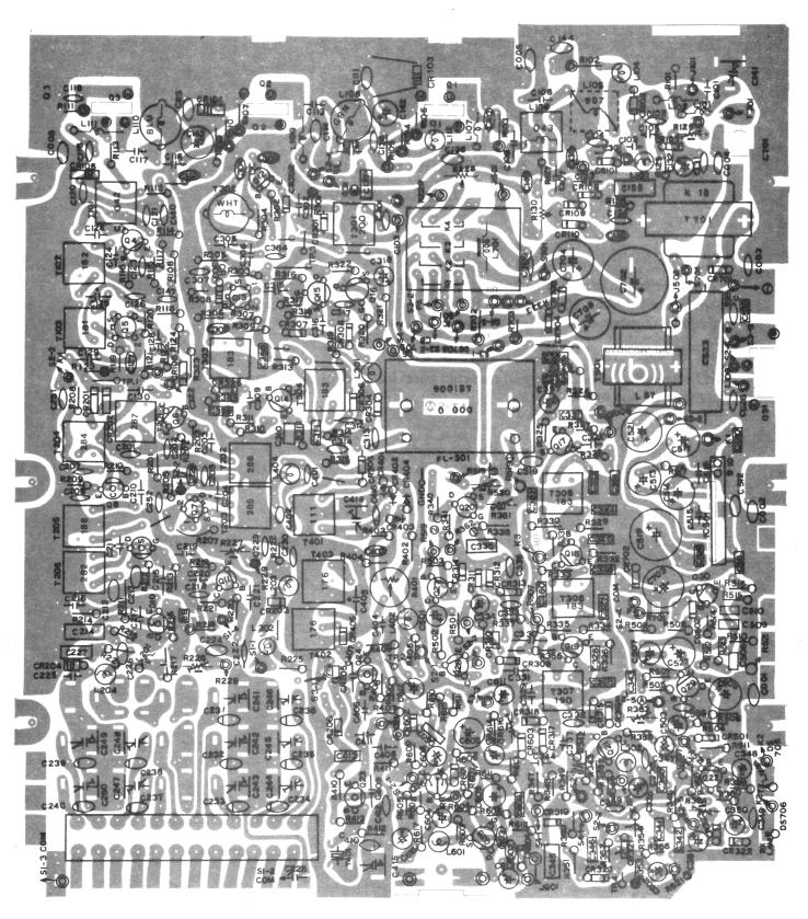
Main Board Parts Locator Both Models (Component Side)
