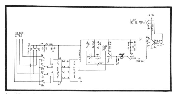
Figure 3-3. Scan Circuit
