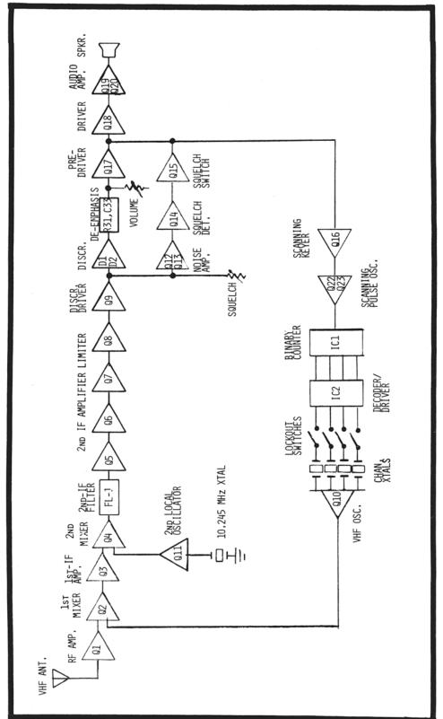
Figure 3-1. Model SCAN 150 Block Diagram
