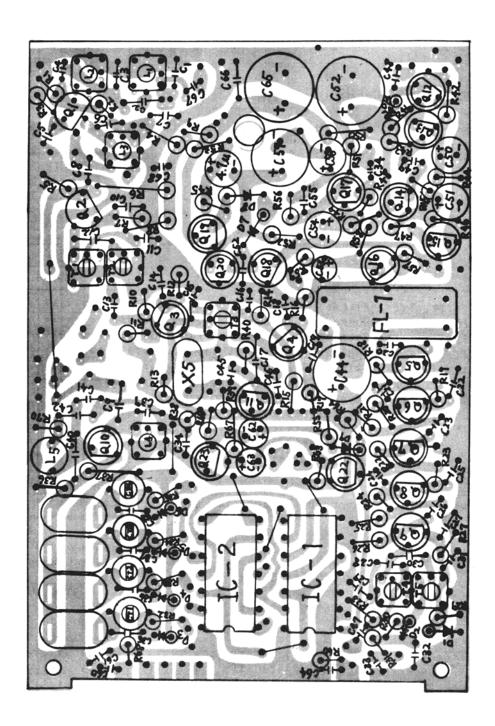
Figure 6-1. Parts Locator (Component Side)
