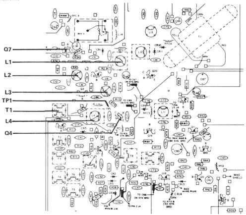
Figure 4-2 Test Point and Adjustment Locations for Receiver Alignment
