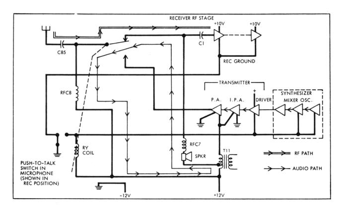
Figure 2-2 Transmit-Receive Switching Schematic
