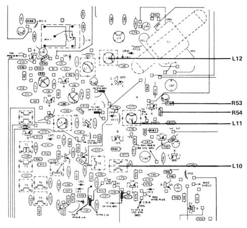
Figure 4-1 Test Point and Adjustment Locations for Transmitter Alignment
