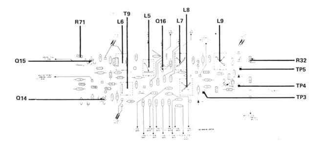
Figure 4-3 Test Point and Adjustment Locations for Synthesizer Board Alignment
