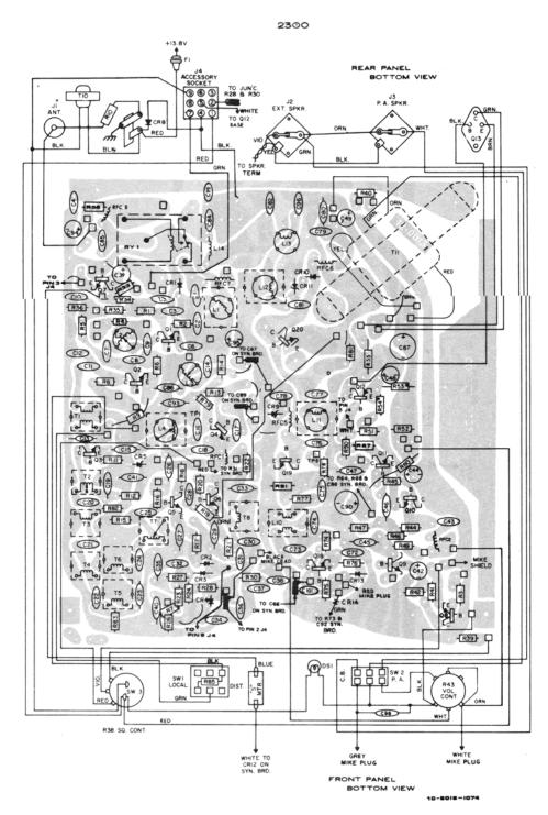
Figure 5-2 Main Board Parts Locator (CB 2300)
