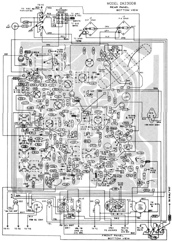
Figure 5-5 Main Board Parts Locator (CB DX2300B)
