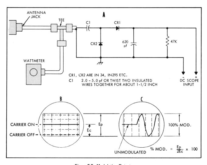
Figure 3-3 Modulation Detector
