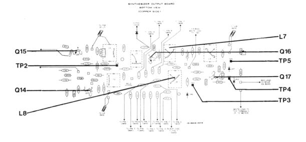
Figure 3-5 Test Point Locations for Transmitter Troubleshooting
