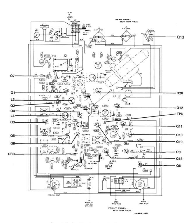
Figure 3-1 Test Point Locations for Voltage Charts
