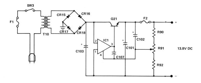
Figure 2-3 Power Supply Circuit
