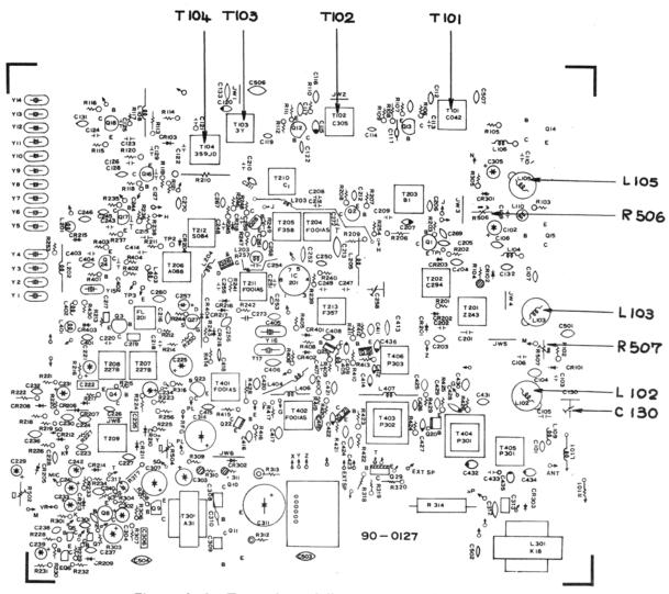
Figure 4-1 Transmitter Adjustment Locations
