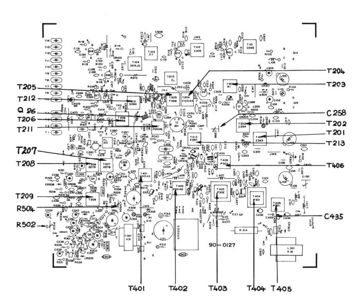
Figure 4-2 Receiver Adjustment Locations
