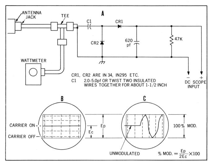
Figure 3-1 Modulation Detector
