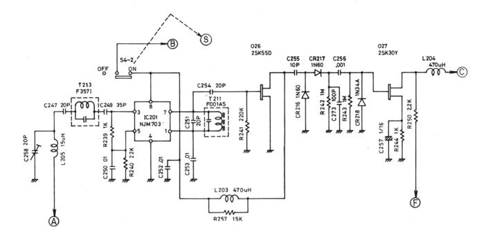
Figure 5-1 Noise Blanking Circuit
