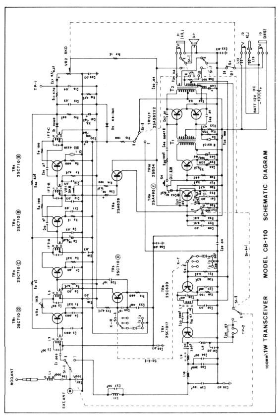
Figure 6-2 CB 110 Schematic
