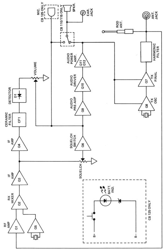
Figure 3-1 CB 110, 115, 125 Block Diagram
