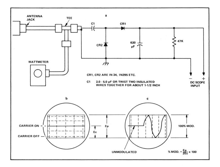
Figure 4-1 Modulation Detector
