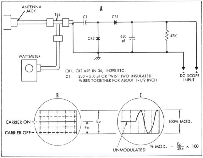
Fig. 2 MODULATION DETECTOR
