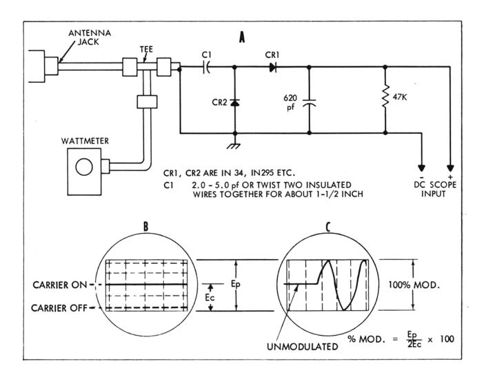
Figure 3-1. Modulation Detector
