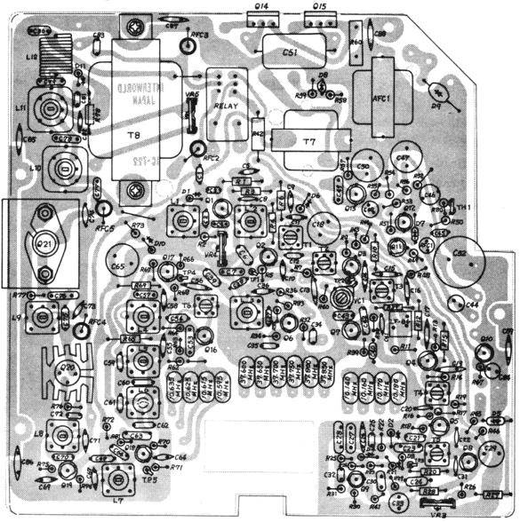
Figure 5-1. Parts Locator (Component Side)
