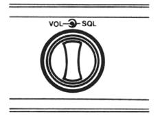
**Step 4:** Turn the power on and adjust the "Volume" control for a satisfactory sound level.
