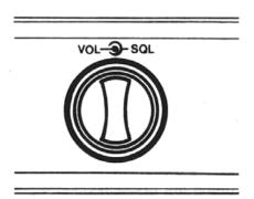
**Step 3:** Make sure the Squelch control is in the 9 o'clock position.
