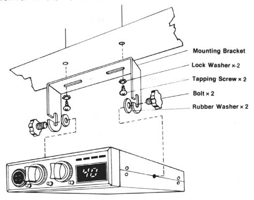
This transceiver may be installed in any 12-volt negative ground-system car or truck. Most current U.S. and foreign vehicles use a negative system.
