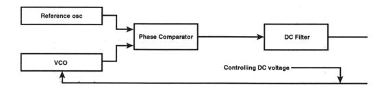
Note in the following that the reference frequency of 2.5 kHz is obtained by dividing the 4.5 MHz by 1800 times. (2,5 kHz reference is used instead of 10 kHz for division convenience).
