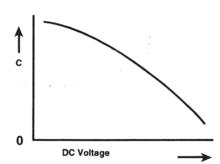
The varactor diode is responsible for setting VCO frequency, and once set it regulates the VCO frequency against the reference.
