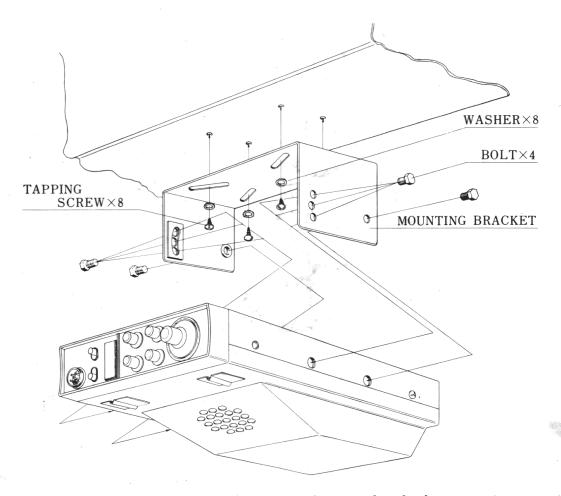
Safety and operating convenience are the primary factors to be considered when mounting any piece of equipment in an automobile. Be sure that the transceiver controls may be easily reached by the operator. Also be sure that connecting cables do not interfere the operation of the brake, accelerator, etc.
