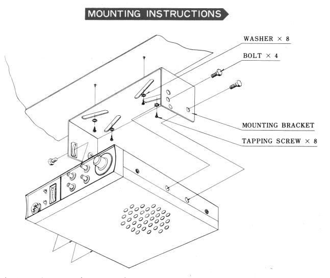
Safety and operating convenience are the primary factors to be considered when mounting any piece of equipment in an automabile. Be sure that the transceiver controls may be easily reached by the operator. Also be sure that connecting cables do not interfere the operation of the brake, accelerator, etc.
