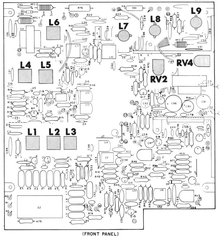
Figure 3-4. Components to be Adjusted for Complete Transmitter Alignment, Stages 3 & 4
