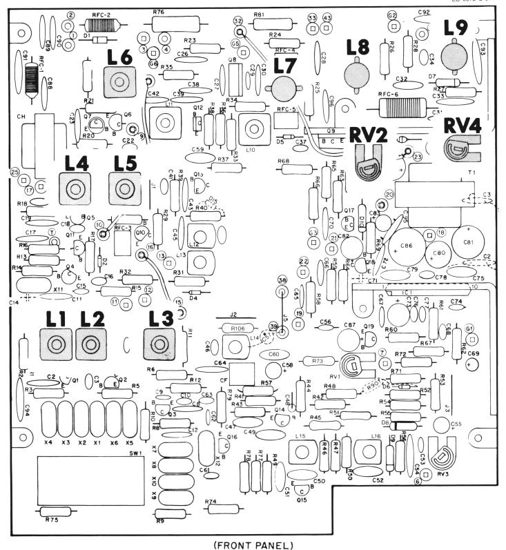
Figure 3-3. Components to be Adjusted for Complete Transmitter Alignment, Stages 1 & 2
