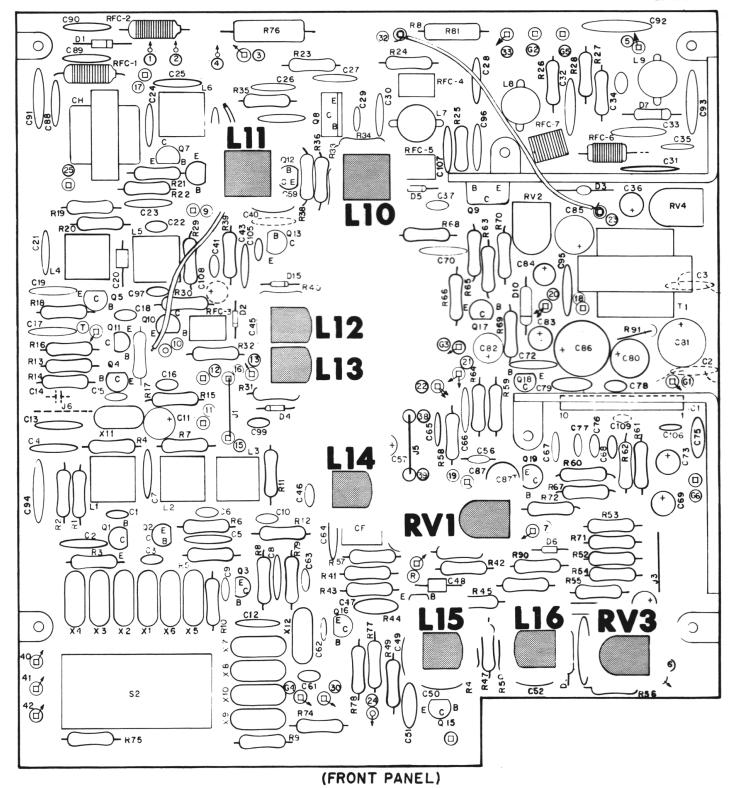
Figure 3-2. Components to be Adjusted for Complete Receiver Alignment, Stages 3 & 4
