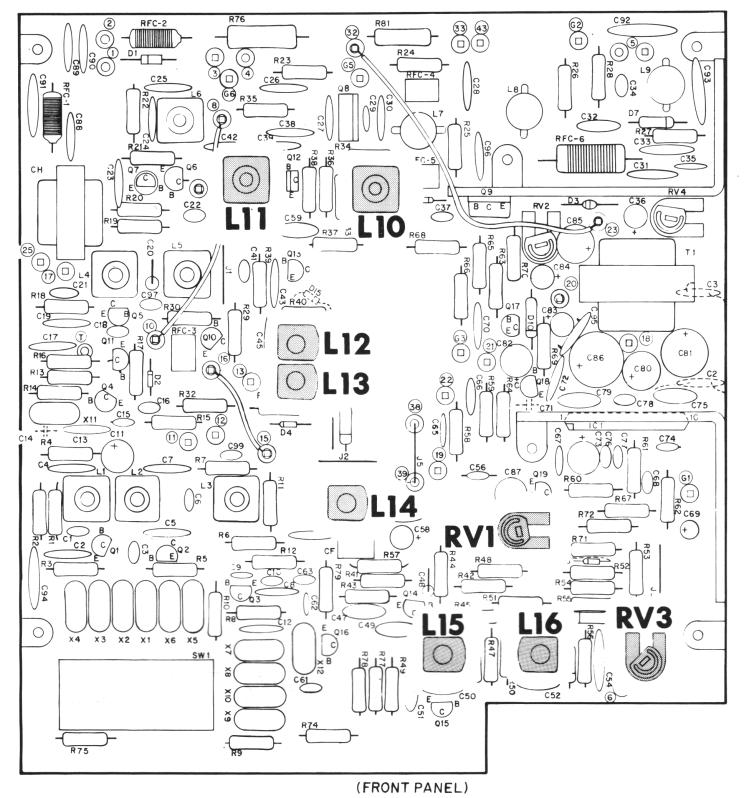
Figure 3-1. Components to be Adjusted for Complete Receiver Alignment, Stages 1 & 2
