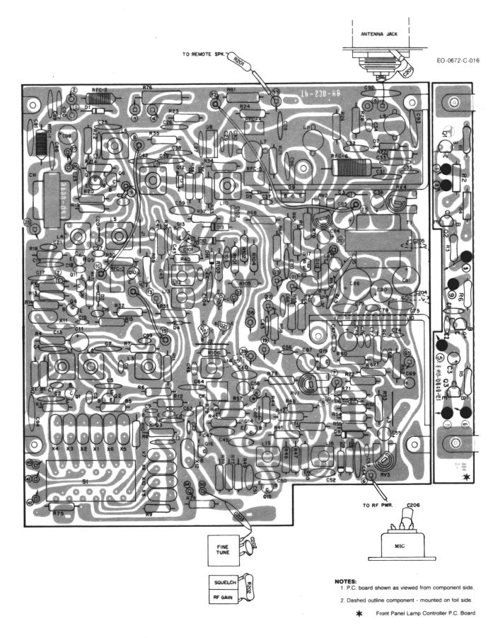
Figure 4-1. P.C. Board, Component Outline, Stage 1
