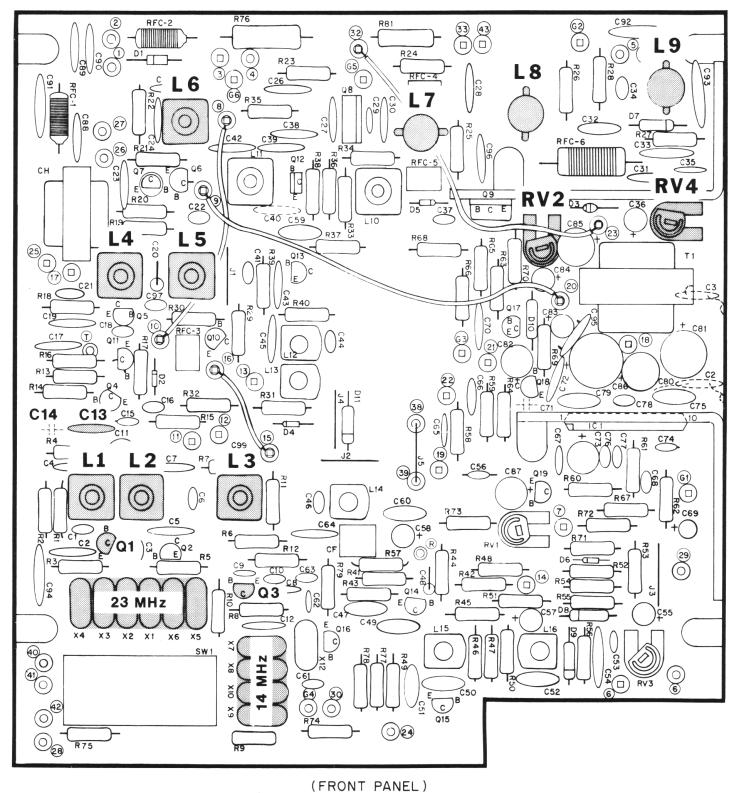
Figure 3-3. Components to be Adjusted for Complete Transmitter Alignment, Stages 1 & 2
