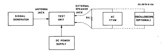
Figure 2-3. Equipment Set-Up, Receiver Alignment
