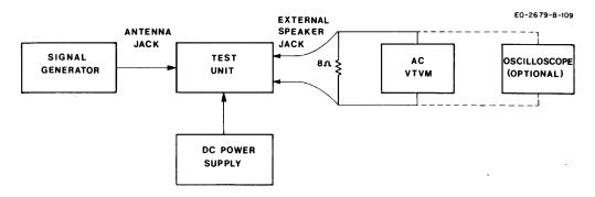
Figure 3-3. Equipment Set-Up, Receiver Alignment
