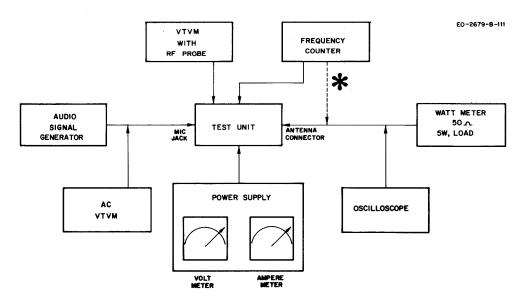
Figure 3-1. Equipment Set-Up, Transmitter Alignment
