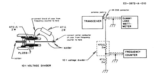
Figure 3-2. Connection of the Frequency Counter and Dummy Load
