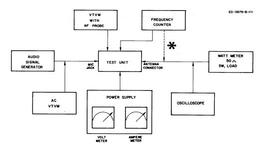
Figure 2-1. Equipment Set-Up, Transmitter Alignment
