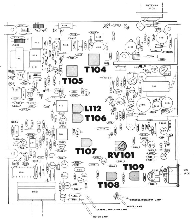
Figure 2-5. Components Adjusted for Receiver Alignment
