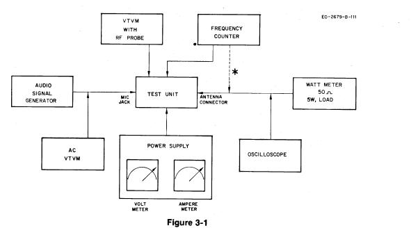
\*NOTE: See Figure 3-2 for connection of the frequency counter and the dummy load.
