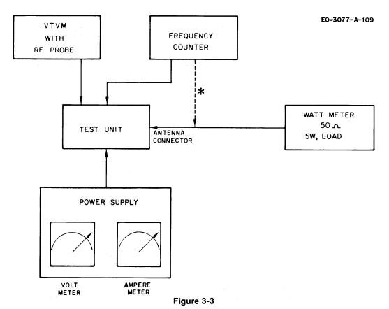
Equipment Set-up, Transmitter Alignment
