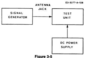
Equipment Set-up, Receiver Alignment
