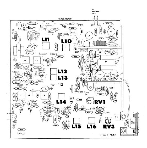
Figure 3-7. Components Adjusted for Receiver Alignment
