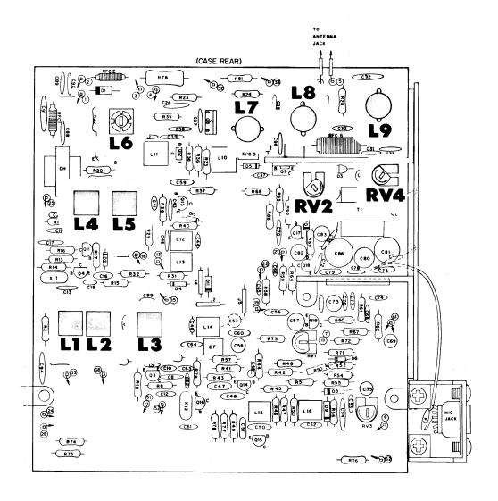
Figure 3-6. Components Adjusted for Transmitter Alignment
