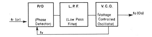
In the above block diagram, when the reference frequency, fr, and the VCO output frequency, fv, are applied to the Phase Detector P/D, fv is compared with fr in terms of phase lag and lead.
