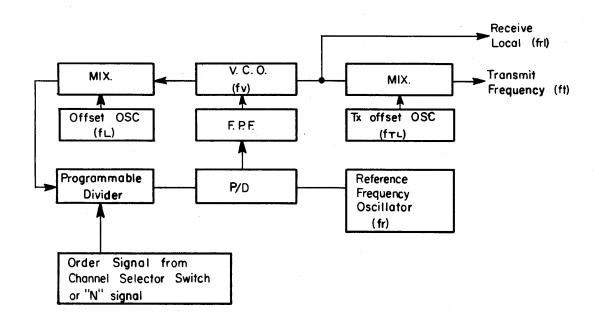
In the block diagram of the synthesizer, the first local oscillator frequency, fRL, for reception, is given below:
