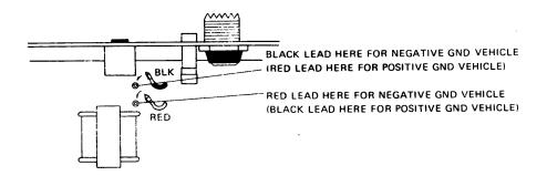
Internal Wiring Change for Positive Ground System
