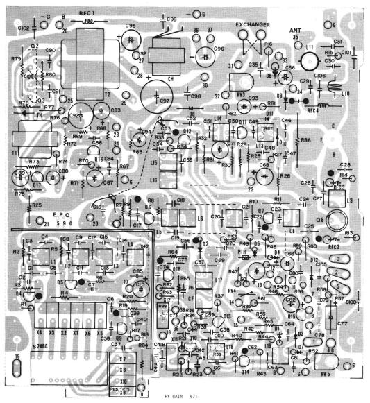
NOTE: 1. R39, R85, R87, R88, C100, C41A, C45 AND C108 ARE MOUNTED ON BOTTOM OF PC BOARD.
