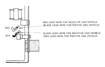
Internal Wiring Change for Positive Ground System
