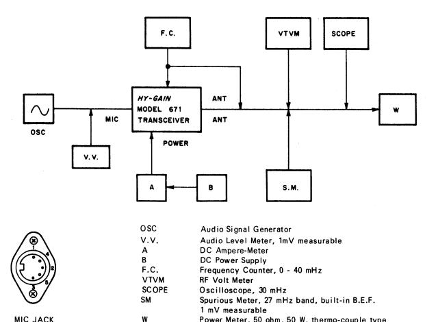
To set the transceiver to transmit mode, connect No. 2 and No. 3 PIN terminals of the DIN type MIC jack to each other by using a wire. When applying modulating signal (MIC input signal), to the unit, connect the signal between the No. 1 and No. 4 (chassis ground) PIN terminals.
