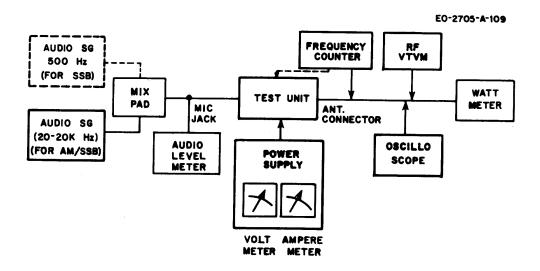
Figure 3-1. Equipment Set-up, Transmitter Alignment
