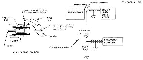
Figure 3-4. Connection of Frequency Counter and Dummy Load
