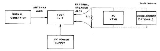
Figure 3-5. Test Equipment Set-Up, Receiver Alignment
