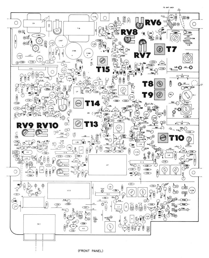
Figure 3-7. Components Adjusted for Receiver Alignment
