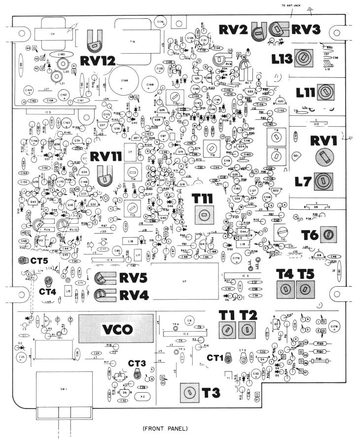
Figure 3-6. Components Adjusted for Transmitter Alignment
