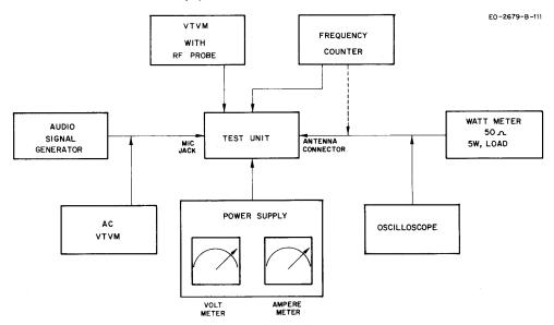
Figure 3-3. Equipment Set-Up for Transmitter Alignment
