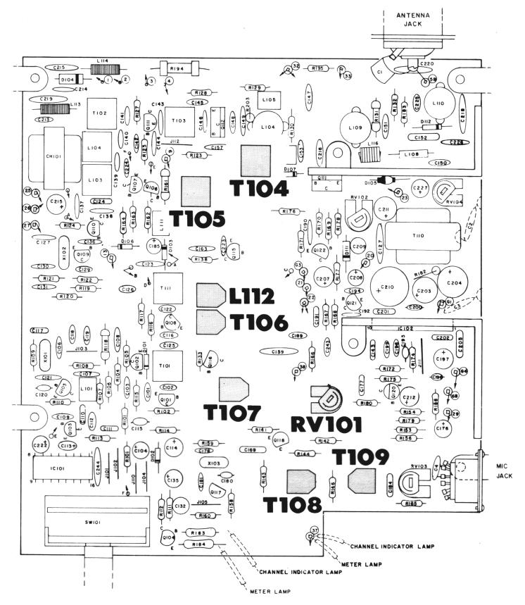
Figure 3-7. Components Adjusted for Receiver Alignment
