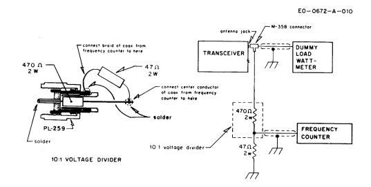
Figure 3-4. Connection of Frequency Counter and Dummy Load
