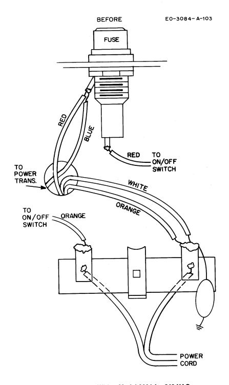
Figure 3-1. Before Wiring Model 3084 for 240 VAC
