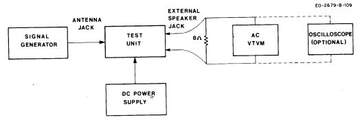
Figure 3-5. Equipment Set-Up for Receiver Alignment
