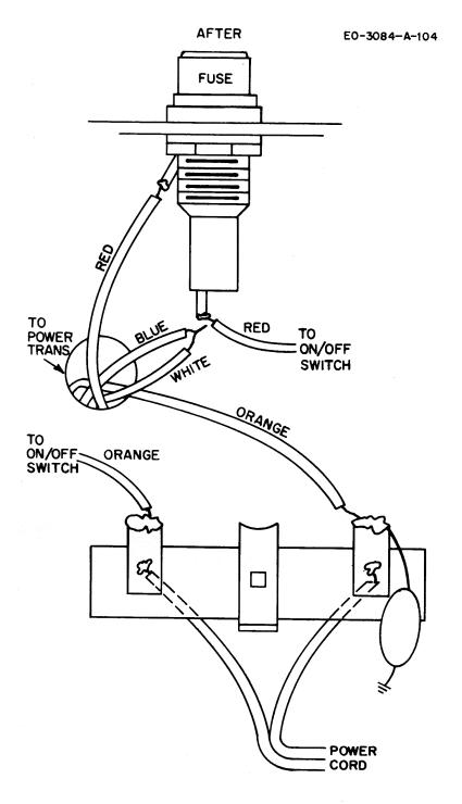
Figure 3-2. After Wiring Model 3084 for 240 VAC
