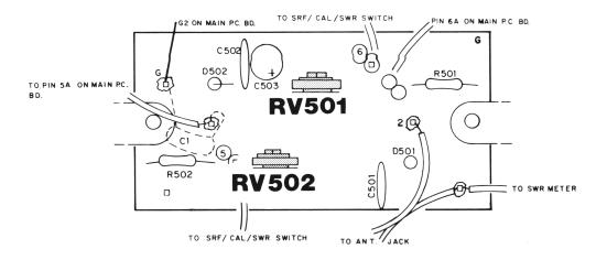
Figure 3-8. Components Adjusted for Meter Alignment
