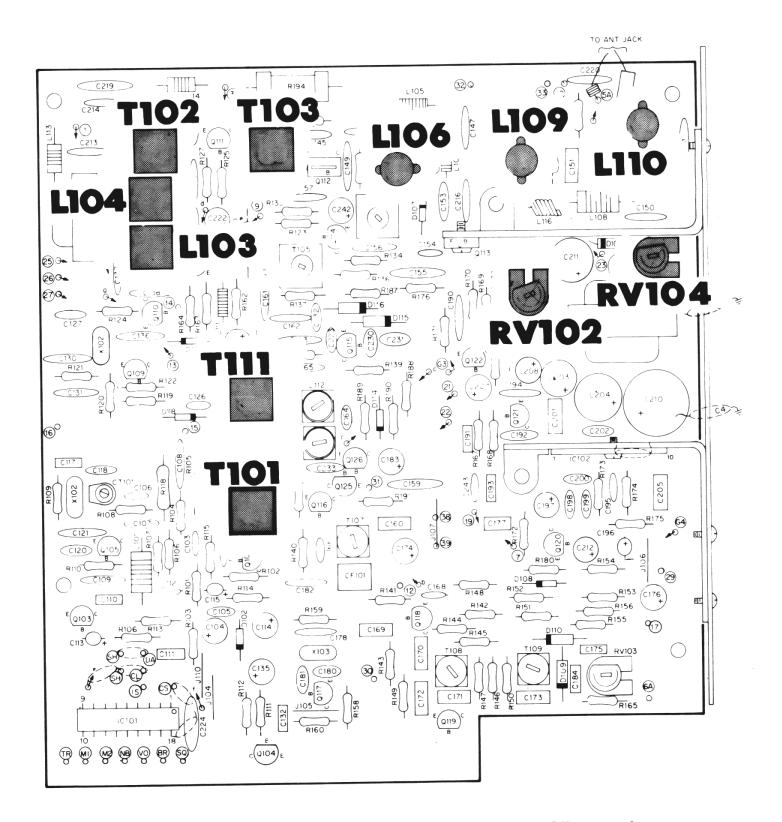
Figure 3-5. Components Adjusted for Transmitter Alignment
