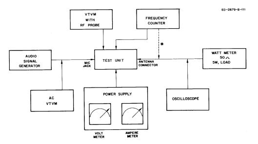
Figure 3-1. Equipment Set-up, Transmitter Alignment
