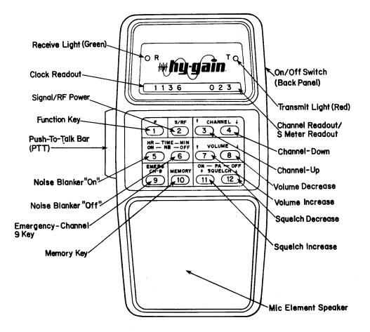
**Figure 1-1. Microphone Controls**
