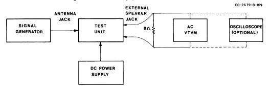
Refer to figure 3-3 for test equipment connection.
