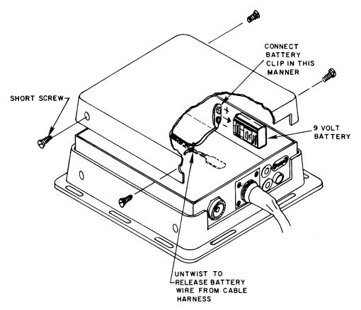
Figure 3-4. Connection of Memory Battery
