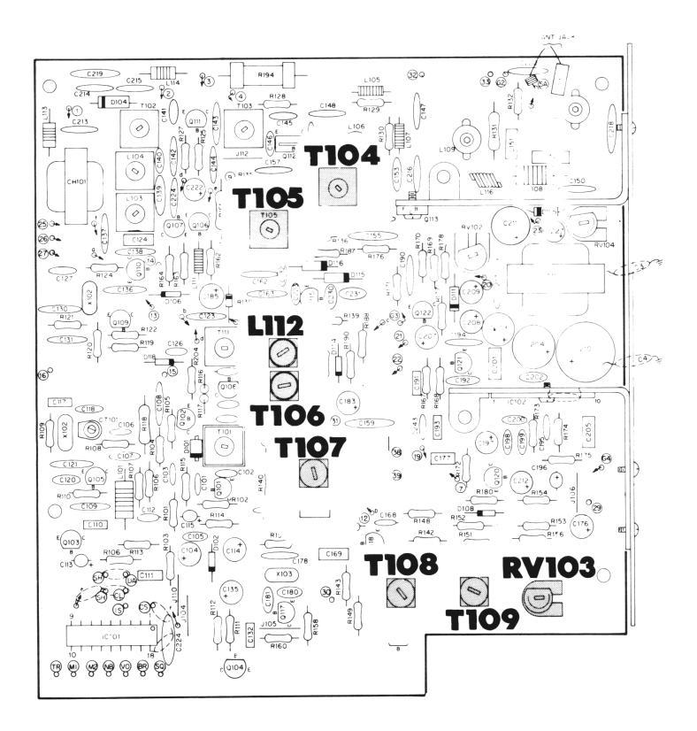
Figure 3-6. Components Adjusted for Receiver Alignment
