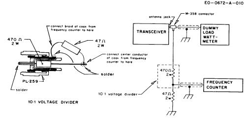
Figure 3-2. Connection of Frequency Counter and Dummy Load to Antenna Jack
