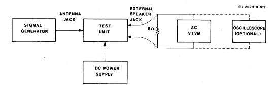
Figure 3-3. Equipment Set-up for Receiver Alignment
