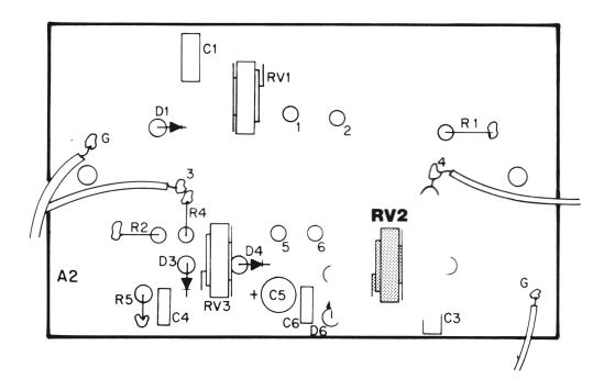
Figure 3-6. Component adjusted for SWR Meter Calibration
