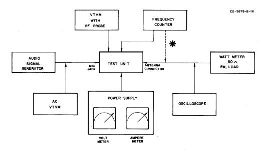
Figure 3-1. Equipment Set-up for Transmitter Alignment
